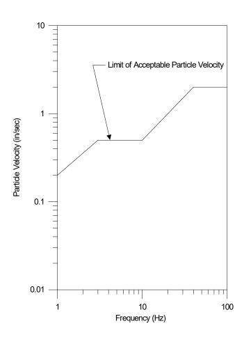
Figure 1 - Vibration Criteria (adapted from AASHTO R8-96)
